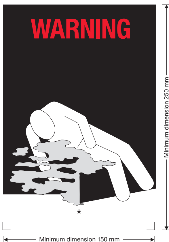
Asphyxiation warning mark for cargo transport units
